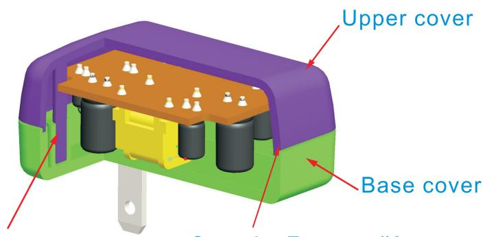
Security Feature #1: Four tight fitted pillars at each corner Security Feature #2: Ultrasonic welding all along the side
